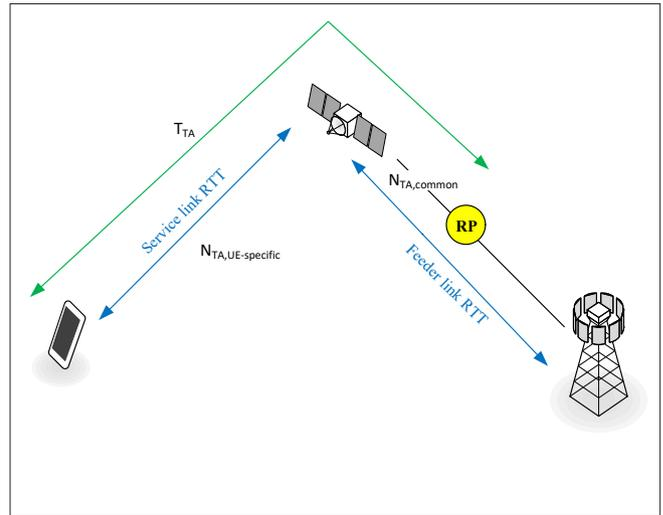
FIGURE 3. Service link RTT, Feeder link RTT, and RP for DL-UL timing alignment.
